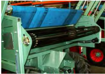
Conveyor belt (featuring removable bars) for highly inclined parcels
