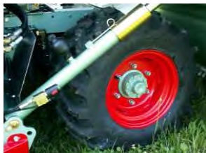
Highly flexible working conditions thanks to the nitrogen shock absorbers
