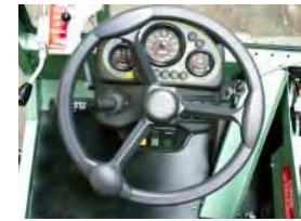
Instrument panel where all controls are within close reach. Optimal visibility of display indicators: petrol level, temperature, engine, milometer, rpm velocity, etc...
