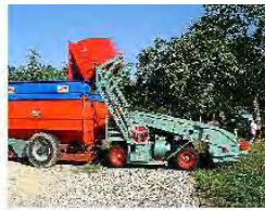
Hopper can be moved in all positions for emptying: in a pit, in a box pallet, in a trailer (2.75 m)
