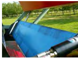
PVC belt facilitates the removal of leaves and branches, for optimal sorting
