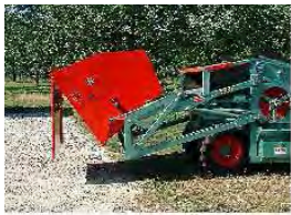
Hopper can be moved in all positions for emptying: in a pit, in a box pallet, in a trailer (2.75 m)
