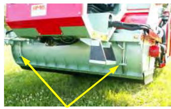
Steel casing in front can be adjusted with two jacks, which helps increase or decrease the machine's hopper size so as to regulate the gathering of fruits, even when a large quantity of leaves is present
