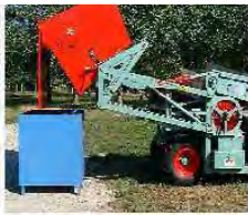
Hopper can be moved in all positions for emptying: in a pit, in a box pallet, in a trailer (2.75 m)
